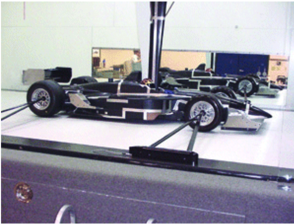
Fig. 1 Typical Indy (Indianapolis Motor Speedway) car model as tested in a wind tunnel. A rolling belt on the floor is used to simulate the moving road. The wheels are mounted separately and rotated by the belt, while the 40%-scale race car's body positioned is changed from above. ( Mark Page; Swift Engineering )
